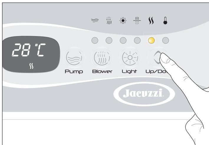
► Press the key "Up/Down" : the display will show the currently memorized temperature, the respective symbol appears and the LED comes on.
