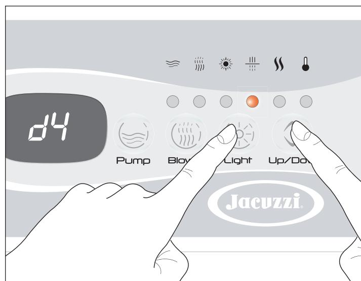
► Press the "Light"
