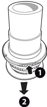
► When carrying out scheduled maintenance, if it is necessary to disassemble the skimmer basket, apply pressure to the relevant area in order to unhook the vessel; therefore disassemble it pushing downwards.
